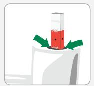
**NOTE:** Create vacuum to green section on gauge. If possible, 'burry' the green so it is no longer visible.
